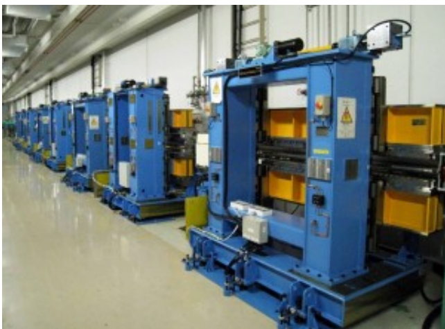
Eight undulators located in the University of Tokyo outstation. © Iwao Matsuda
