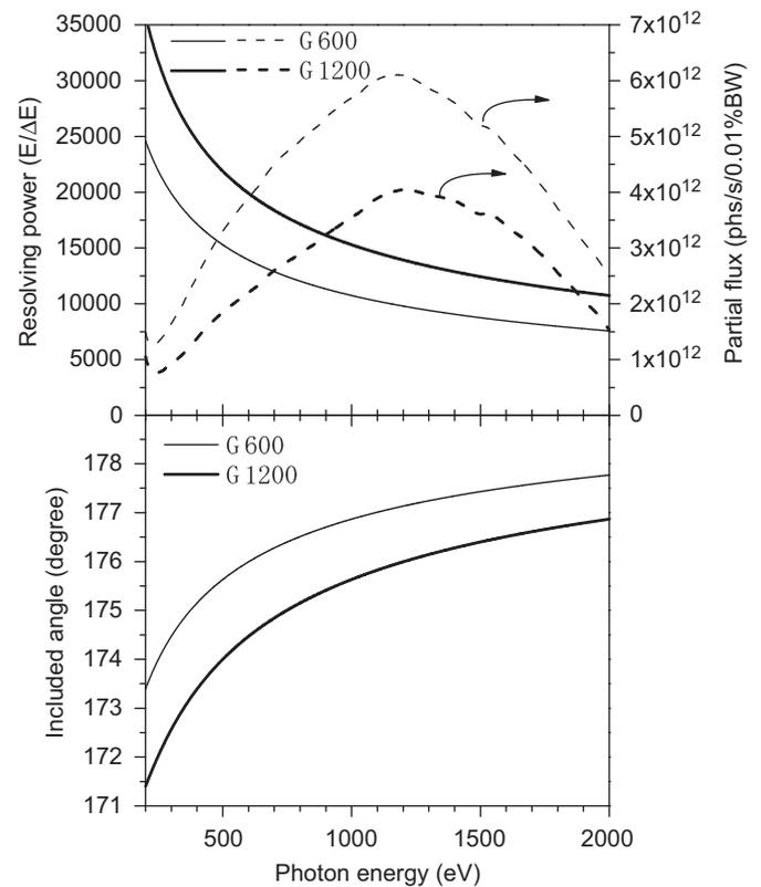
Fig. 2. Calculated energy resolving power, photon flux at exit slit and optimized included angle for G600 (solid line) and G1200 (bold line). Energy resolving power is calculated with an exit slit width of 25  $\mu\text{m}$ . Photon flux is calculated with front end slit opening of 2 mm  $\times$  2 mm.
