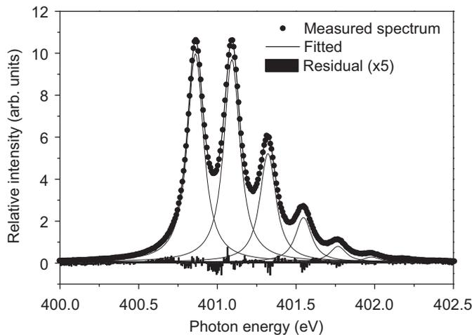
Fig. 3. Total-ion yield spectrum of  $N_2$  at the  $N 1s \rightarrow \pi^*$  region.
