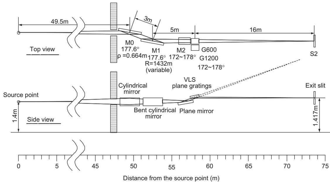
Fig. 1. Optical layout of BL07LSU at Spring-8.
